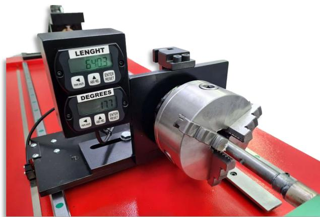
Length and rotation measuring system with digital display
