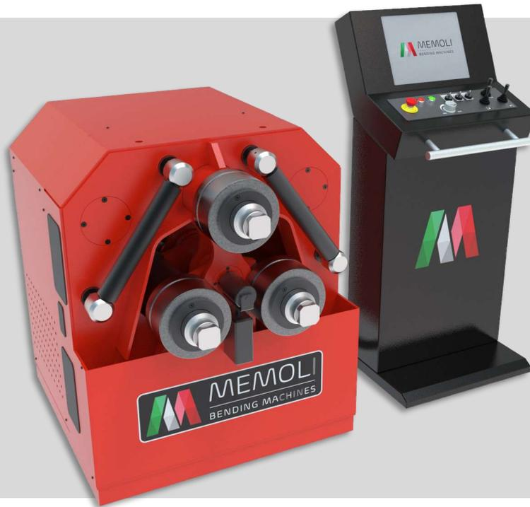
The MEK 60-R **three-roll hybrid profile bender** was designed to meet the demands of an increasingly demanding Customers base, with the need to bend all types of profiles and tubes with **accuracy** and very tight tolerances. The three driving rolls are driven by a powerful electric gearmotor that guarantees high positioning accuracy, while the independent planetary movement of the two bottom rolls is provided by two powerful hydraulic cylinders.
