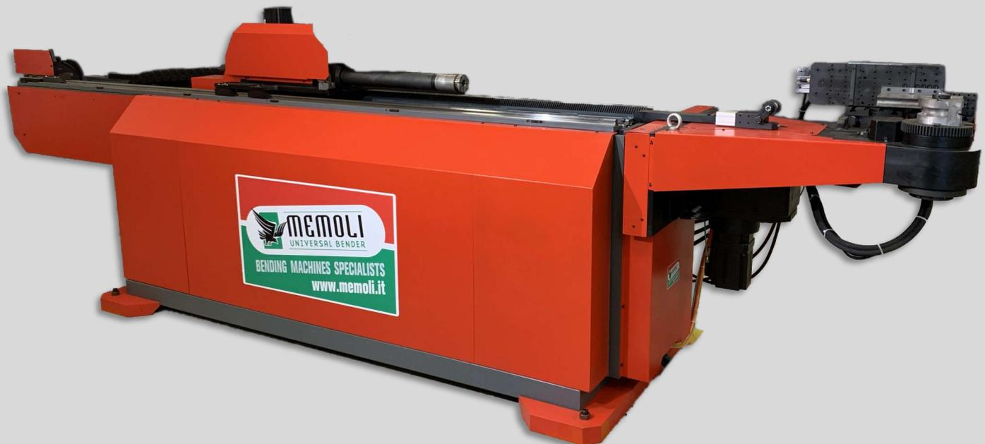
The ACH range is the series of **3-axis CNC bending machines** for the linear bending of tubes up to 65 mm diameter. The bending machines of the ACH series are fully automatic bending machines with CNC 3 axes: **bending** (Y axis), **advancement** (X axis) and **rotation** (Z axis).
