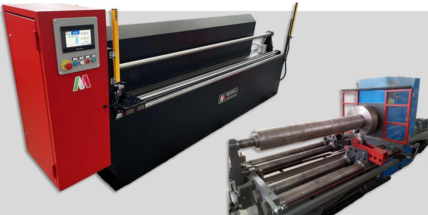
The HLN series of coiling lathes are *full electric CNC-controlled machines* designed for the manufacture of springs and augers. Designed and built entirely by Memoli, they are an effective and efficient solution capable of machining round, flat, square bars and tubes.
