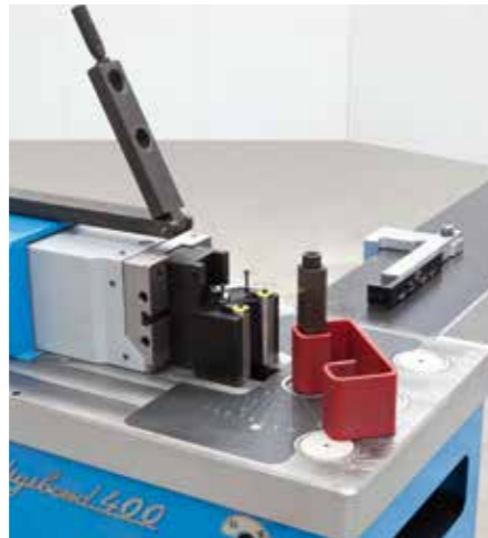
Bending tool with pin \varnothing 50 mm, H=200 mm, revolving pin single V die and antiflection bar. max. 200 x 8 mm. Patent Pending.
