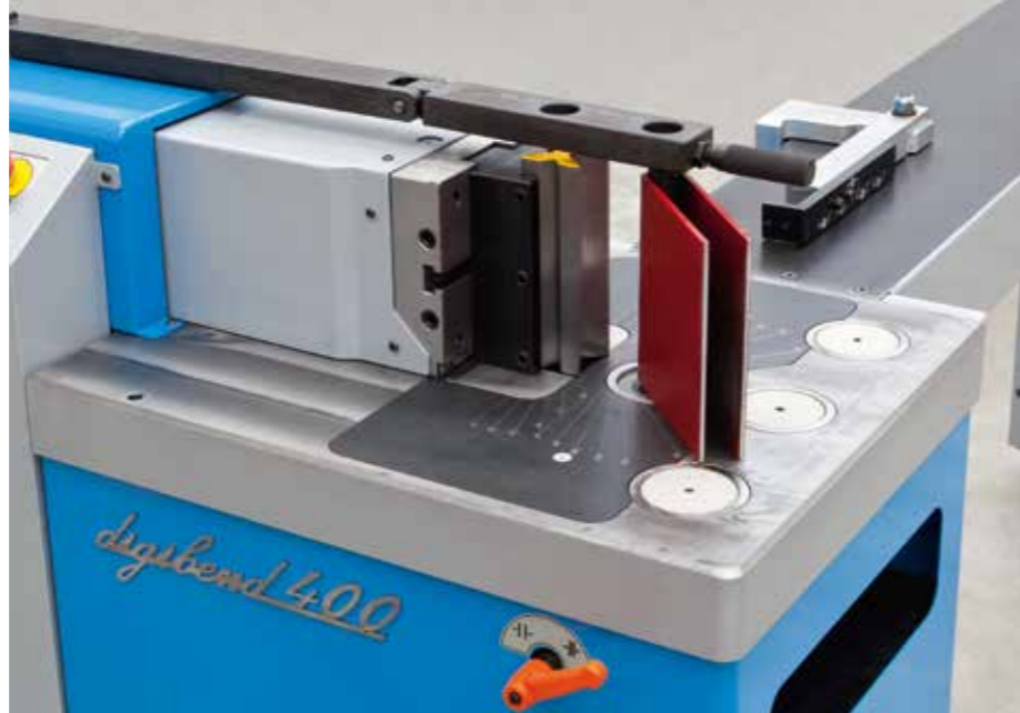
Bending tool with pin \varnothing 30 mm, H=200 mm and antiflection bar. Max 200 x 5 mm.
