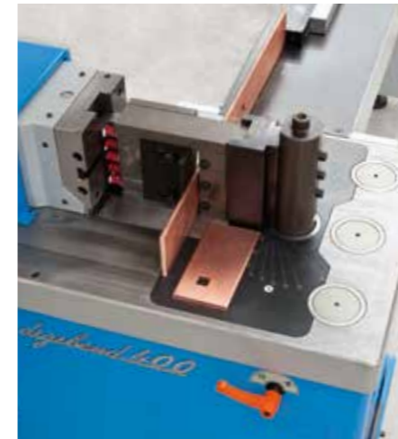
Shearing unit for flat bars. Max 150 x 12 mm.
