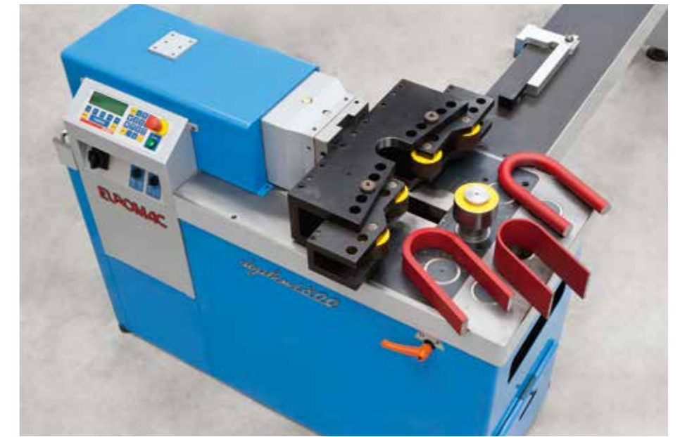
4 jaw bending tool for round, square, rect. bars and thick pipes up to 180°. Max 100 x 20 mm or \varnothing 50 mm.
