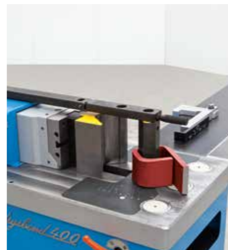
Pin bending punch \varnothing 80 mm with antiflection bar for bending a closed loop into thick wall bars. Max 200 x 15 mm.
