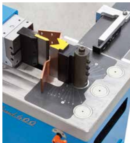
Movable bending punch and fixed die for tight bends.
