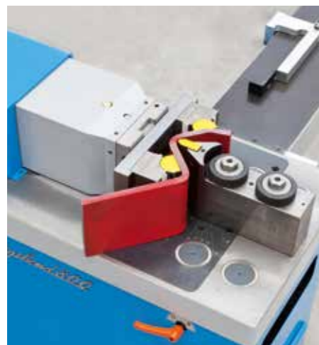
Tool single V die with revolving pin (mark-free bending) for thick plates. Max 200 x 40 mm.
