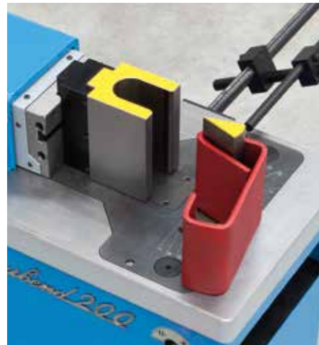
Bending tool 30° with U shaped die for bending flat bars up to 30°. Max. 16 x 200 mm.
